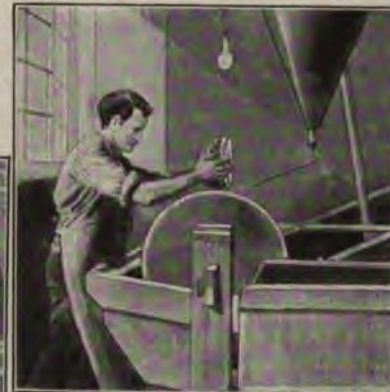
3. Glass vessels are pressed into shape and then cut on a revolving stone, as shown in the picture.
